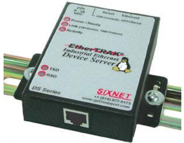
Compact Size with DIN Rail Mounting Standard
