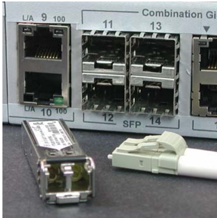
This image shows a typical SFP/LC transceiver and dual-LC cable.
