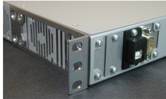
In the image above, the brackets are mounted flush with the back of the switch.
