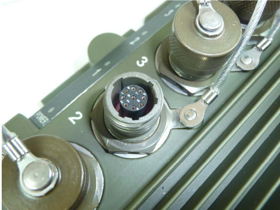
Ethernet Receptacle Location (typical)
